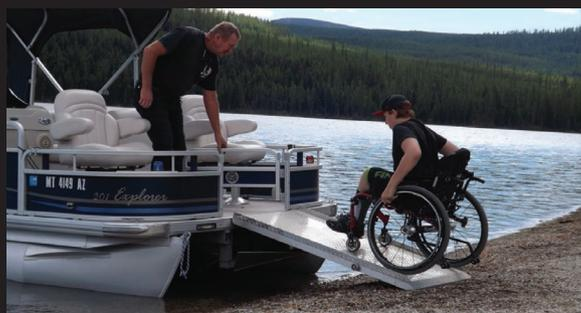
**SELF DEPLOYING PONTOON BOAT RAMP**
